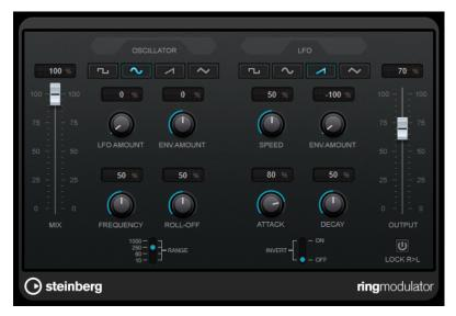
Ring modulators work by multiplying two audio signals. The ring-modulated output contains added frequencies generated by the sum of, and the difference between, the frequencies of the two signals.
