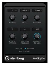
Gating, in its fundamental form, silences audio signals below a set threshold. If a signal rises above the set level, the gate opens to let the signal through. Signals below the set level are silenced. **MidiGate**, however, is not triggered by threshold levels, but MIDI notes. Therefore, it needs both audio and MIDI data to function.
