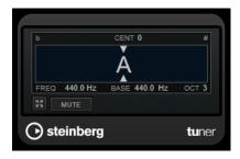
The graphical display indicates the currently played pitch as a note. The two arrows indicate any pitch deviation. The deviation is also shown in the upper area of the display. If the played note is flat of the pitch, the pitch indicator is located to the left. If the played note is sharp, the pitch indicator is located to the right.
