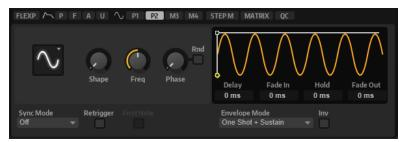
You can adjust the times of the envelope in the graphical editor by dragging nodes left or right.
