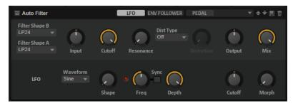
Morphing between the two shapes, as well as the cutoff, can be controlled with a manual pedal control, an LFO, or an envelope follower.
