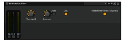
Due to its fast attack time, Brickwall Limiter can reduce even short audio level peaks without creating audible artifacts. However, this plug-in creates a latency of 1 ms. Brickwall Limiter features separate meters for input, output, and the amount of limiting.
