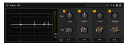
With the four frequency bands, you can shape the tone color, to create a brighter or darker sound, for example. The two mid-range bands act as peak filters, and the low and high bands act as shelving filters. All bands are fully parametric with adjustable gain, frequency, and Q factor. Each frequency band offers the following controls:
