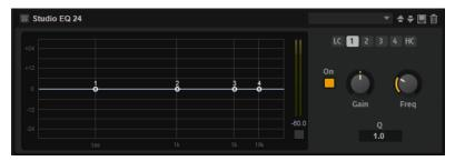
Click one of the numbered buttons to show the settings for the corresponding frequency band. The two mid-range bands act as peak filters, and the low and high bands act as shelving filters. Each frequency band offers the following controls:
