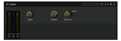
The input and output meters indicate the level before and after the Limiter. The Gain Reduction meter in the middle indicates the current attenuation of the level.
