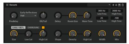
The early reflections are responsible for the spatial impression in the first milliseconds of the reverb. For emulating different rooms, you can choose from different early reflection patterns and adjust their size. The reverb tail, or late reverberation, offers parameters for controlling the room size and the reverb time. You can adjust the reverb time individually in three frequency bands.
