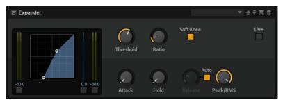
The graphical control to the left shows the expansion curve. You can edit the **Threshold** and **Ratio** values with the handles of this control. The input and output meters indicate the level before and after the expansion. The Gain Reduction meter indicates the current attenuation of the level.
