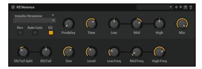
By recording an impulse in a room, you capture the characteristics of this room. Convolution superimposes these characteristics on the sound. The result is a very authentic reverb.
