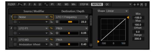
The modulation matrix offers you up to 32 freely assignable modulations, each with a source, an offset parameter, a modifier, and a destination with adjustable depth. All modulation sources and destinations can be assigned several times. The polarity of each source can be switched
