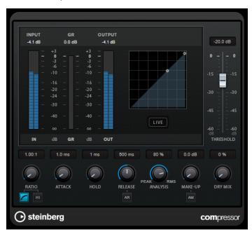
**Compressor** features a separate display that graphically illustrates the compressor curve that is shaped according to the **Threshold** and **Ratio** parameter settings. **Compressor** also features a **Gain Reduction** meter that shows the amount of gain reduction in dB, **Soft knee/Hard knee** compression modes, and a program-dependent auto feature for the **Release** parameter.
